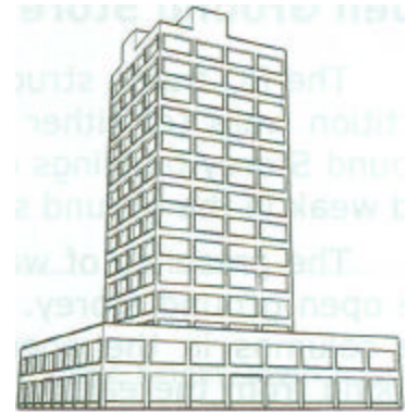
R.C. frame structure with Podium
